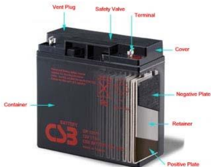
Figure 1: Construction of VRLA battery
